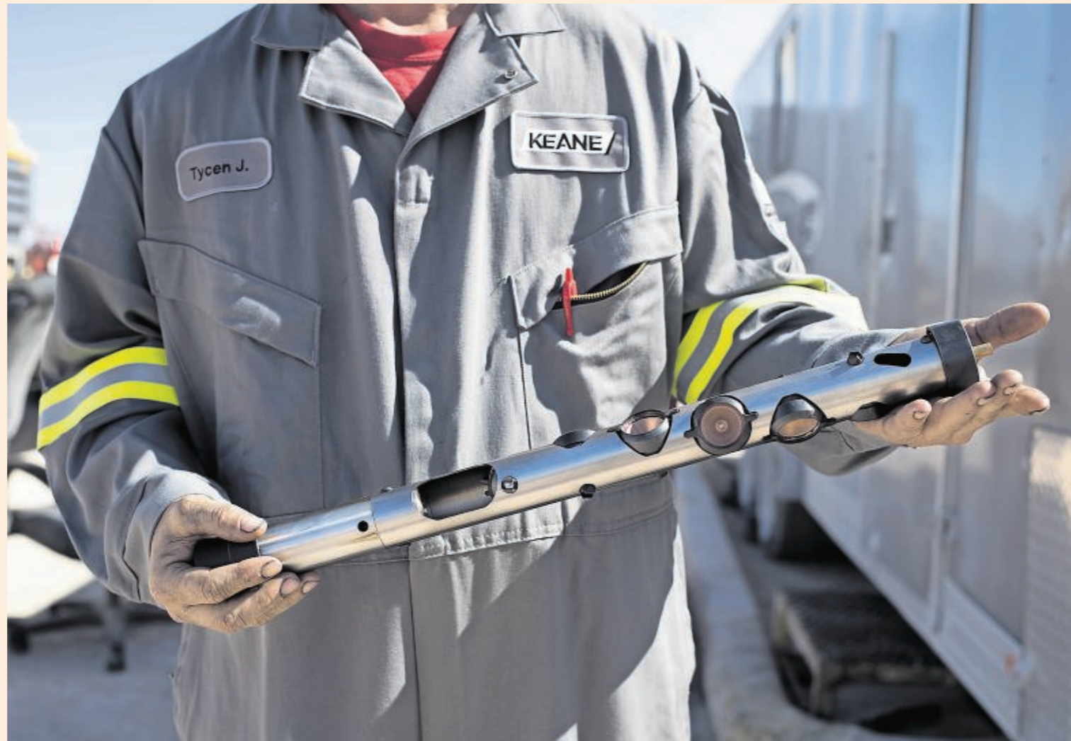
A Royal Dutch Shell worker holds a hydraulic fracturing perforating gun, used to penetrate shale rock — Matthew Busch/Bloomberg
